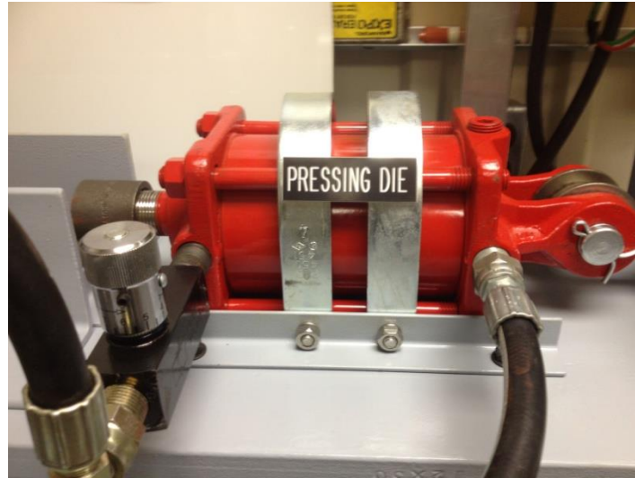
Figure 4.25 Horizontally mounted hydraulic cylinder for pressing force
