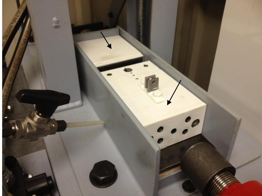
Figure 4.42 Thermally insulated pressing and clamping dies placed in manufacturing unit
