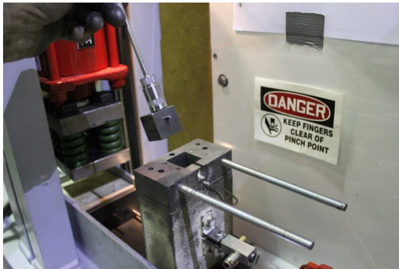
Figure 4.15 Die insert being removed from holding block with a hand held magnet tool during processing
